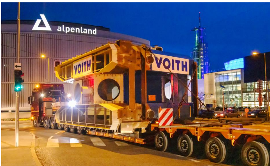
Special transport of the 6.5m wide turbine housing from St. Poelten to the Ziller Valley in Tyrol
