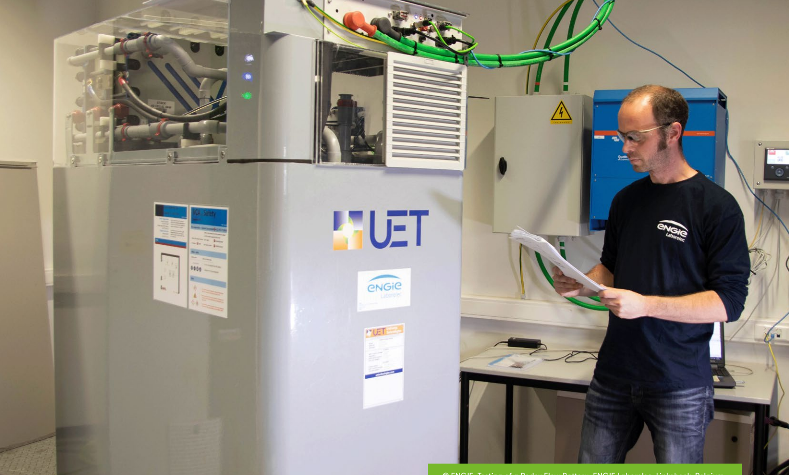
© ENGIE, Testing of a Redox Flow Battery, ENGIE Laborelec, Linkebeek, Belgium.
