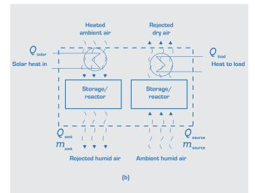
Open-cycle adsorption system
