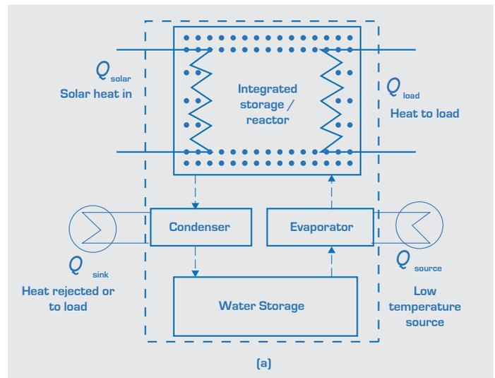
Closed-cycle adsorption system
