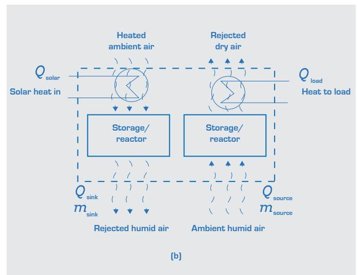
Open-cycle adsorption system
